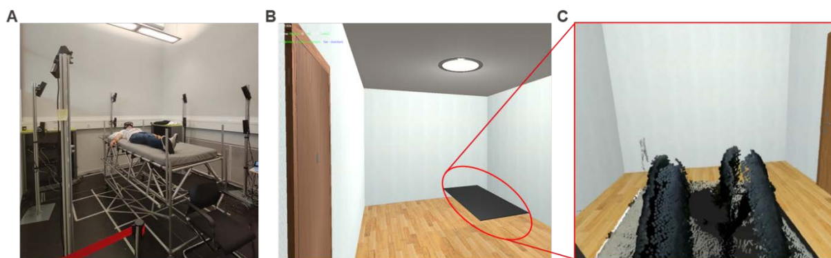
Figure 1. Experimental setup and virtual environment. Using ten Kinect cameras around a participant (A), appearance parameters of the body and of the objects surrounding the body are transferred to the virtual environment (B) as a photorealistic avatar or photorealistic virtual objects. Inside the virtual environment, the participant can see the virtual body and the virtual objects from a body-centered viewpoint (C). Also, movements of the virtual body are synchronized with these of the physical body. The black plate in (B) is the location of the virtual bed and the virtual body.
