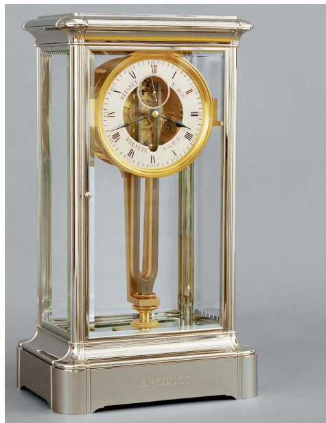
Figure 1.3 – Louis-Clément Breguet’s 1867 tuning fork clock with a frequency of 100 Hz (Musée International d’Horlogerie, La Chaux-de-Fonds).
