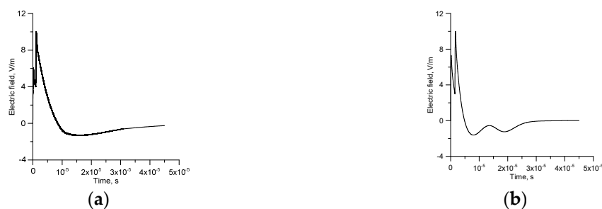
Figure 13. The effect of multiple streamer bursts arising from the same origin on the NBP. In the simulation, the growth parameters of each streamer burst is assumed identical to the one used previously except that the value of n_0 was selected to make the peak of the NBP equal to 10 V/m at 100 km. (a) separation between streamer bursts 1.0 \mu\text{s} ; (b) separation between streamer bursts 1.5 \mu\text{s} .
