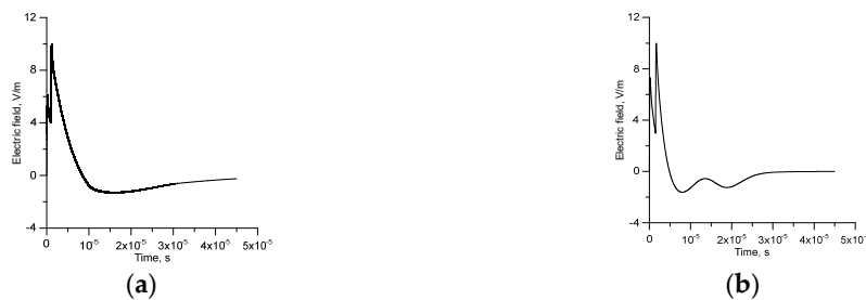
Figure 13. The effect of multiple streamer bursts arising from the same origin on the NBP. In the simulation, the growth parameters of each streamer burst is assumed identical to the one used previously except that the value of n_0 was selected to make the peak of the NBP equal to 10 V/m at 100 km. (a) separation between streamer bursts 1.0 \mu s; (b) separation between streamer bursts 1.5 \mu s.
