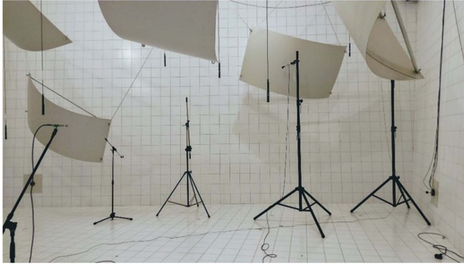
Figure 10. Measurement set up in a real reverberation chamber in the laboratory.
