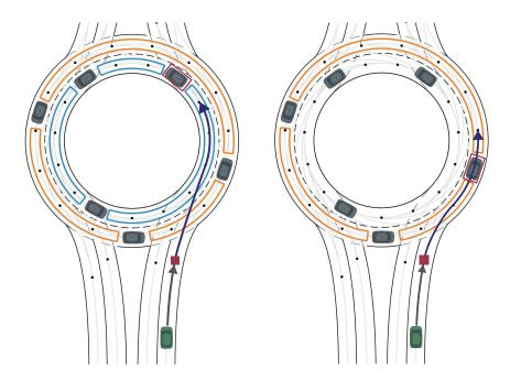
Figure 4.4 – Illustration of two eligible maneuver candidates to perform a merging maneuver into a two-lane roundabout, whose reference path is shown by the blue arrow and its currently safe portion is shown in gray. Inter-vehicle gaps belonging to different subsets are shown in different colors. Filled square represents the decision spot. The vehicles framed in a red box represent the relevant obstacles encoded within the maneuver candidates.
