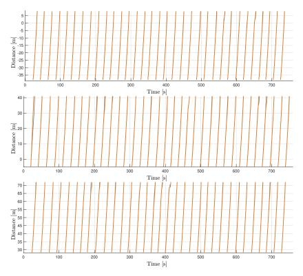
Figure 8.9 – Time-distance diagrams representing the evolution of the incoming traffic in every incoming lane in the simulated scenario  $16R1LR3L1I10-100V-500Q[1\ 1\ 1]$ . The trajectories of R-Agents and PR-Agents are represented by (  $\_$  ) and (  $\_$  ), respectively.
