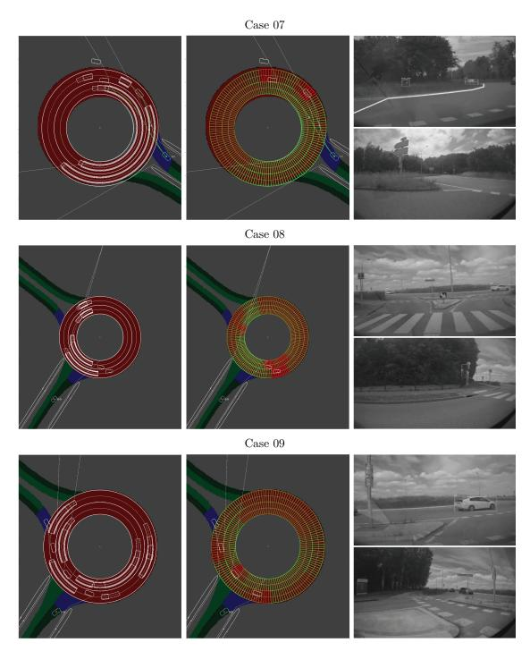
Figure 9.8 – Representation of the probably-free gaps extraction at three different times (one case per row). Cases 7-9. From left to right: state of the DOG representing the occupancy probability distribution of the circulatory lanes, representation of the extracted gaps, footage of two cameras in the vehicle's front bumper.
