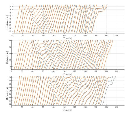
Figure 7.15 – Time-distance diagrams representing the evolution of the incoming traffic in every incoming lane in the simulated scenario  $16R1LR3L1I10-100V-2500Q[1\ 1\ 1]$ . The trajectories of R-Agents and IC-Agents are represented by (  $\_$  ) and ( $\_$  ), respectively.
