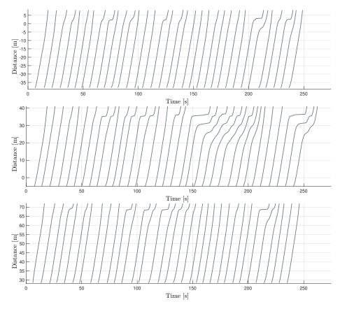
Figure 5.7 – Time-distance diagrams representing the evolution of the incoming traffic in every incoming lane in the simulated scenario  $16R1LR3L1I10-100V-1500Q[1\ 1\ 1]$ .
