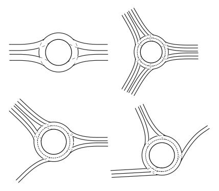
Figure 2.3 – Four examples of roundabout geometries that can be automatically generated with our simulation platform. Among examples we have varied the number of circulatory lanes, the number of legs, and the number of incoming and outgoing lanes in each leg.
