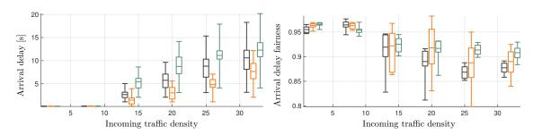
Figure 5.14 – On the left-hand side, boxplots representing the distribution of arrival delay for different incoming traffic inflow volumes and configurations. On the right-hand side, the fairness with which the arrival delay is distributed among the vehicles in the scenarios.
