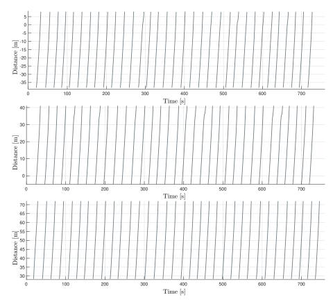
Figure 5.4 – Time-distance diagrams representing the evolution of the incoming traffic in every incoming lane in the simulated scenario  $16R1LR3L1I10-100V-500Q[1\ 1\ 1]$ .
