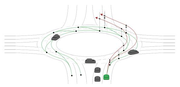
Figure 4.1 – Illustration of the motion planning task. The green vehicle represents the ego vehicle. The two red lines represent two possible trajectories the ego vehicle could follow, whose elevation (vertical displacement) represent time. The set of green lines and dots plotted on the road represent a lane-graph showing some path alternatives that would allow the ego vehicle to drive through the intersection.
