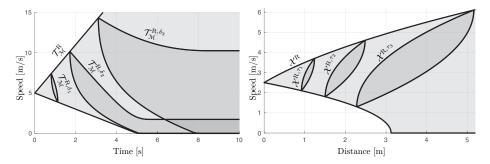
Figure 8.2 – On the left-hand side, illustration of three sets of reachable maneuver targets, given an initial state  $x_0 = (0, 5)$ , and for distances  $\delta = \{1, 3, 5\}$  to three hypothetical decision spots; along with their envelope set. On the right-hand side, illustration of three sets of reachable states for three different time intervals and initial state  $x_0 = (0, 2.5)$ .
