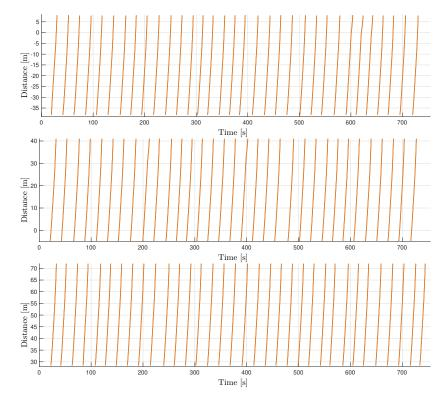
Figure 7.9 – Time-distance diagrams representing the evolution of the incoming traffic in every incoming lane in the simulated scenario  $16R1LR3L1I10-100V-500Q[1\ 1\ 1]$ . The trajectories of R-Agents and IC-Agents are represented by ( — ) and ( — ), respectively.
