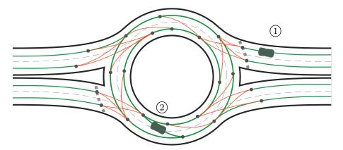
Figure 4.3 – Lane-graph representation of a two-lane roundabout. Segments ( $\longrightarrow$ ) represent car-following edges, while segments ( $\longrightarrow$ ) show the gap-acceptance ones.
