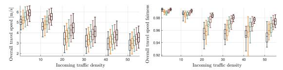
Figure 8.18 – On the left-hand side, boxplots representing the distribution of overall travel speed applied by the vehicles for different incoming traffic inflow configurations and penetration rates. On the right-hand side, the fairness with which the metric is distributed among the vehicles in the scenarios.
