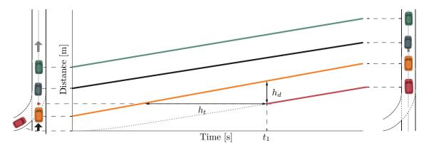
Figure 2.13 – Time-distance diagram representation.
