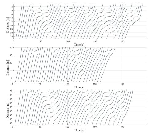
Figure 5.10 – Time-distance diagrams representing the evolution of the incoming traffic in every incoming lane in the simulated scenario 16R1LR3L1I10-100V-2500Q[1 1 1].
