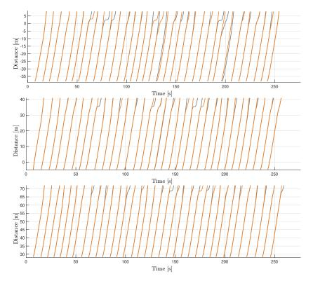
Figure 7.12 – Time-distance diagrams representing the evolution of the incoming traffic in every incoming lane in the simulated scenario  $16R1LR3L1I10-100V-1500Q[1\ 1\ 1]$ . The trajectories of R-Agents and IC-Agents are represented by ( — ) and ( — ), respectively.
