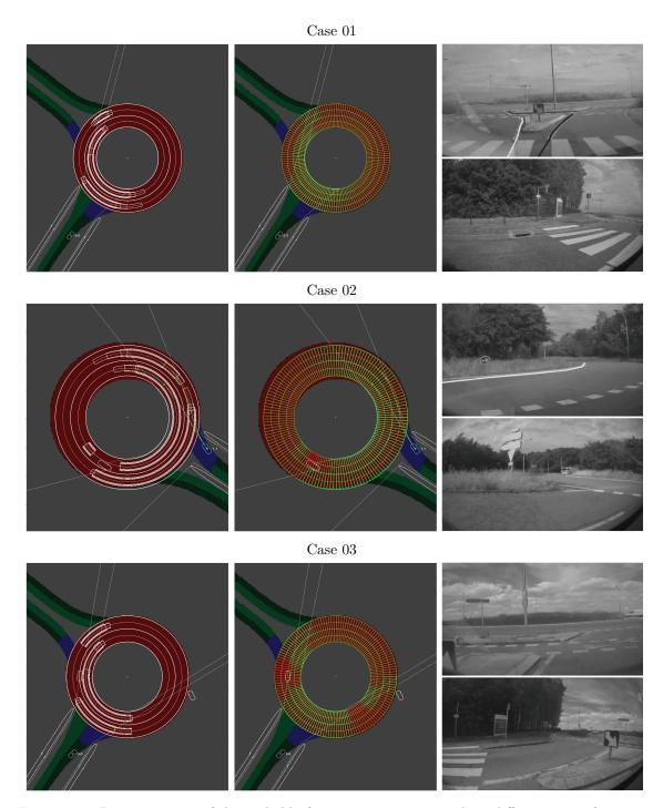
Figure 9.6 – Representation of the probably-free gaps extraction at three different times (one case per row). Cases 1-3. From left to right: state of the DOG representing the occupancy probability distribution of the circulatory lanes, representation of the extracted gaps, footage of two cameras in the vehicle's front bumper.
