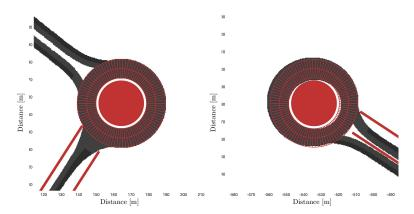
Figure 9.4 – Representation of the two roundabouts in the experimental scenario, along with the fitted occupancy grid, and the considered environmental obstacles.
