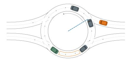
Figure 7.2 – Illustration of the example scenario. The green vehicle represents the ego vehicle, who intends to facilitate the merging maneuver of the orange vehicle. The inter-vehicle gap highlighted in orange, represents the gap the ego vehicle has control over, hence the one it would try to modify so that the orange vehicle merges into it.
