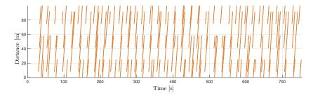
Figure 7.8 – Time-distance diagram representing the evolution over time of the vehicles in the circulatory lane, in the simulated scenario 16R1LR3L1I10-100V-500Q[1 1 1]. The trajectories of R-Agents and IC-Agents are represented by ( — ) and ( — ), respectively.
