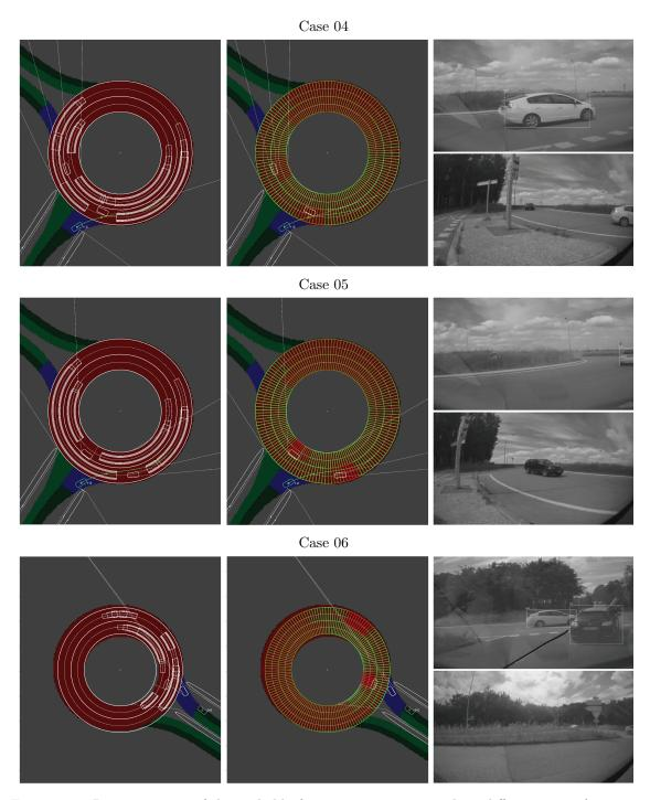
Figure 9.7 – Representation of the probably-free gaps extraction at three different times (one case per row). Cases 4-6. From left to right: state of the DOG representing the occupancy probability distribution of the circulatory lanes, representation of the extracted gaps, footage of two cameras in the vehicle's front bumper.
