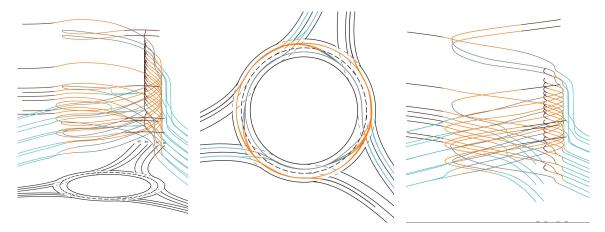
Figure 2.12 – Three-dimensional representation of the trajectories followed by a set of vehicles driving through a roundabout. Time is represented in the vertical axis.
