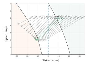
Figure 7.6 – Example of the evolution of the gap in the example scenario, when the minimum cooperative deceleration feasible is applied. The color code used represents in ( — ) the gap's states that would not be accepted, and in ( — ) the ones that would.
