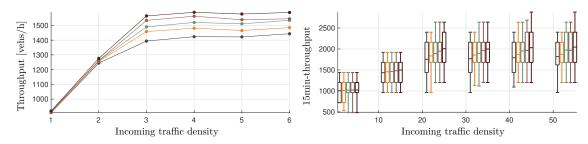
Figure 6.21 – On the left-hand side, the total intersection throughput registered for different incoming traffic density, and values of the penetration rate of EC-agents. On the right-hand side, boxplots representing the distribution of 15min-throughput for different incoming traffic inflow configurations and penetration rates.
