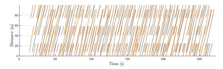
Figure 8.11 – Time-distance diagrams representing the evolution of the incoming traffic in every incoming lane in the simulated scenario 16R1LR3L1I10-100V-1500Q[1 1 1]. The trajectories of R-Agents and PR-Agents are represented by ( — ) and ( — ), respectively.
