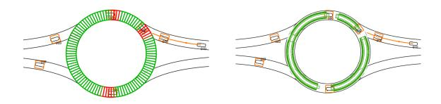
Figure 2.7 – On the left-hand side, debugging view where the path of the vehicle of interest, the objects it detects, and the state of the intersection it perceives is shown. On the left-hand side, an additional debugging representation showing the inter-vehicle gaps the pinned vehicle observes are shown.
