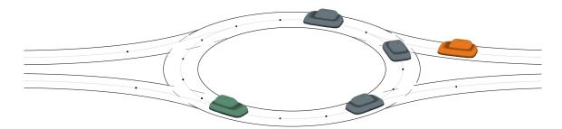
Figure 7.1 – Illustration of the addressed traffic scenario. The green car represents an AV that is evaluating its options regarding behaving cooperatively with the orange vehicle, which is the subject of the cooperation.
