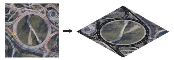
Figure 2.4 – Illustration of the process to manually create a roundabout layout. On the left-hand side, the top view of the roundabout and a set of Bézier curves defined by the user. On the right-hand side, screenshot of a simulation based on the resulting geometry. Roundabout image obtained from maps.google.com
