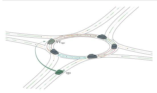
Figure 6.1 – Illustration of the problem tackled by the communication-based maneuver planner. The ego vehicle is represented by the merging green vehicle. In the circulatory lane, the translucent vehicle represents the virtual vehicle the ego vehicle projects in the circulatory lane, so that such location is reserve for it to perform its merging maneuver.
