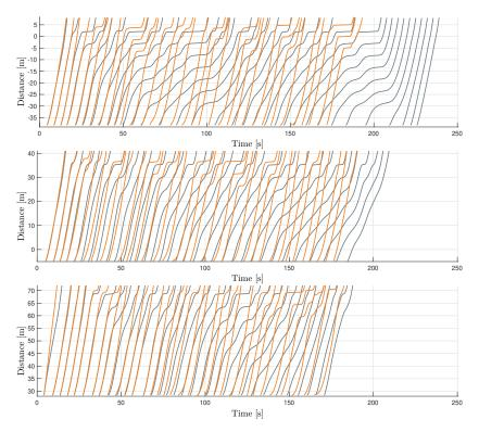
Figure 8.15 – Time-distance diagrams representing the evolution of the incoming traffic in every incoming lane in the simulated scenario  $16R1LR3L1I10-100V-2500Q[1\ 1\ 1]$ . The trajectories of R-Agents and PR-Agents are represented by ( — ) and ( — ), respectively.
