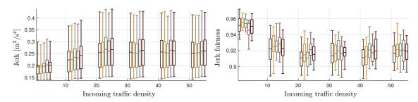
Figure 7.19 – On the left-hand side, boxplots representing the distribution of jerk for different incoming traffic inflow volumes and configurations. On the right-hand side, the fairness with which the jerk is distributed among the vehicles in the scenarios.
