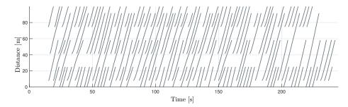
Figure 5.9 – Time-distance diagrams representing the evolution of the incoming traffic in every incoming lane in the simulated scenario  $16R1LR3L1I10-100V-2500Q[1\ 1\ 1]$ .
