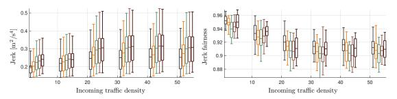
Figure 8.19 – On the left-hand side, boxplots representing the distribution of jerk for different incoming traffic inflow volumes and configurations. On the right-hand side, the fairness with which the jerk is distributed among the vehicles in the scenarios.
