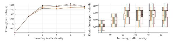
Figure 7.20 – On the left-hand side, the total intersection throughput registered for different incoming traffic density, and values of the penetration rate of IC-agents. On the right-hand side, boxplots representing the distribution of 15min-throughput for different incoming traffic inflow configurations and penetration rates.
