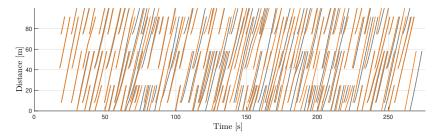
Figure 7.11 – Time-distance diagram representing the evolution over time of the vehicles in the circulatory lane, in the simulated scenario  $16R1LR3L1I10-100V-1500Q[1\ 1\ 1]$ . The trajectories of R-Agents and IC-Agents are represented by (  $\longrightarrow$  ) and ( $\longrightarrow$ ), respectively.
