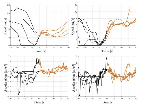
Figure 9.3 – Examples of the speed and acceleration merging profiles registered in each of the roundabouts in the scenario. Segments ( $\longrightarrow$ ) represent positions out of the roundabout, while ( $\longrightarrow$ ) correspond to instants where the ego vehicle is inside either of the roundabouts.
