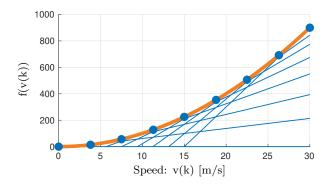
Figure 4.6 – Illustration of the convexification process used to formulate the original non-linear safety constraint as a set of linear inequalities.
