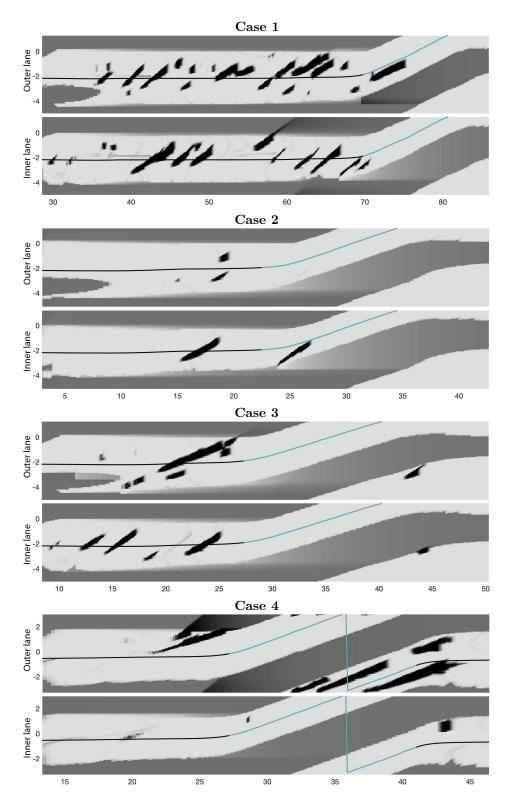
Figure 9.5 – Samples of the evolution of the DOG representing the occupancy state of the circulatory lanes, in four different scenarios registered in the provided data set.
