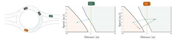
Figure 10.3 – On the left-hand side, a roundabout scenario. In the middle, gap-acceptance decision map used by the green vehicle to decide when to merge into the roundabout. On the right-hand side, the gap-acceptance decision map that the orange vehicle would use to determine if it could cooperate with the green vehicle.
