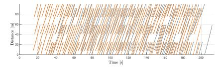
Figure 7.14 – Time-distance diagram representing the evolution over time of the vehicles in the circulatory lane, in the simulated scenario  $16R1LR3L1I10-100V-2500Q[1\ 1\ 1]$ . The trajectories of R-Agents and IC-Agents are represented by (  $\longrightarrow$  ) and (  $\longrightarrow$  ), respectively.
