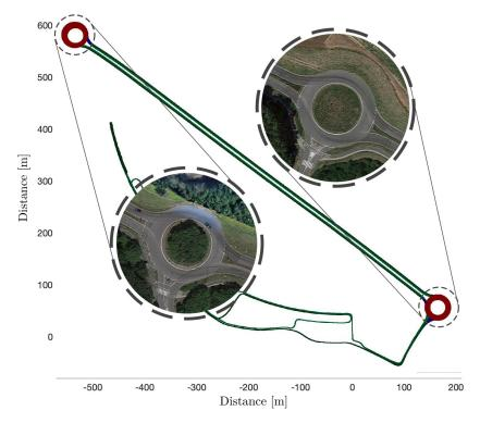
Figure 9.1 – Map of the scenario where the experiments take place. Green pixels represent lanes where the ego vehicle is allowed to drive. Red pixels show positions inside the surrounding roundabouts. Blue pixels, found in the incoming lanes to the roundabout, show the areas where the ego vehicle could expect to find fully stopped vehicles, and would be allowed to fully stop itself.
