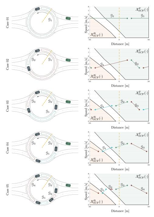
Figure 5.2 – Examples of the decision resulting from the application of the proposed self-serving reactive maneuver planner in a set of five traffic scenes (one case per row). The representation follows the same structure than 5.1.
