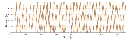
Figure 8.8 – Time-distance diagram representing the evolution over time of the vehicles in the circulatory lane, in the simulated scenario 16R1LR3L1I10-100V-500Q[1 1 1]. The trajectories of R-Agents and PR-Agents are represented by ( — ) and ( — ), respectively.
