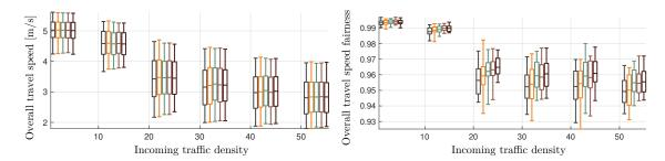
Figure 7.18 – On the left-hand side, boxplots representing the distribution of overall travel speed for different incoming traffic inflow volumes and configurations. On the right-hand side, the fairness with which the overall travel speed is distributed among the vehicles in the scenarios.
