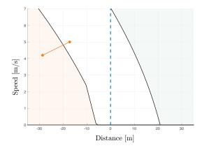
Figure 7.3 – Illustration of the *gap-acceptance decision map* corresponding to the merging trajectory the circulatory vehicle in Fig. 7.2 would presume approaching vehicles apply (see Section 5.3.3 for details on the gap-acceptance decision map). Moreover, the state of the gap ahead of the ego vehicle in Fig. 7.2 is represented by the orange segment. As the gap does not bridge the two sets of the gap-acceptance map, the current state of the gap would not be accepted.
