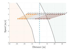
Figure 7.4 – Decision map of the presumed merging trajectory, and the evolution of a gap whose limits move at constant speed. The color code used represents whether: ( $\longrightarrow$ ) only the gap's rear limit, ( $\longrightarrow$ ) neither of the gap's limits, and ( $\longrightarrow$ ) only the gap's front limit would be considered safe by the merging vehicle.
