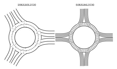
Figure 2.9 – Two roundabout scenarios illustrating the roundabout geometry we consider. On the left-hand side, a 20R2LR3L2I20 roundabout. On the right-hand side, a 50R3LR4L3I30 roundabout.
