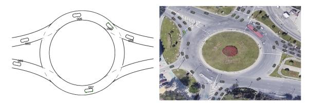
Figure 2.6 – Examples of the two on-line visualizations options our simulation environment supports. On the left-hand side, a two dimensional on-line representation. On the right-hand, a three dimensional view with the real image the roundabout's geometry is extracted from placed in the background.
