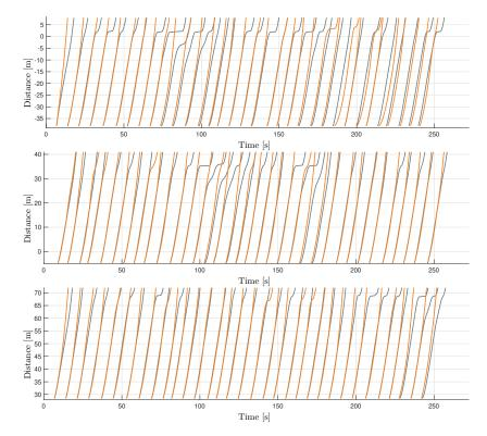
Figure 8.12 – Approaching vehicles' time-distance trajectory resulting from predictive-reactive planning in the scenario. 16R1LR3L1I10-100V-1500Q[1 1 1]. The trajectories of R-Agents and PR-Agents are represented by ( — ) and ( — ), respectively.
