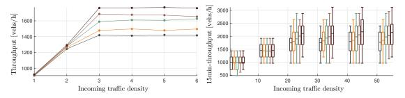
Figure 8.20 – On the left-hand side, the total intersection throughput registered for different incoming traffic density, and values of the penetration rate of PR-agents. On the right-hand side, boxplots representing the distribution of 15min-throughput for different incoming traffic inflow configurations and penetration rates.
