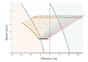
Figure 7.5 – Evolution of the gap in the example scenario when the maximum cooperative deceleration is applied. Colors represent whether:  $( \ \_\ )$  only the gap's rear limit,  $( \ \_\ )$  both of the gap's limits, and  $( \ \_\ )$  only the gap's front limit would be considered safe by the merging vehicle.
