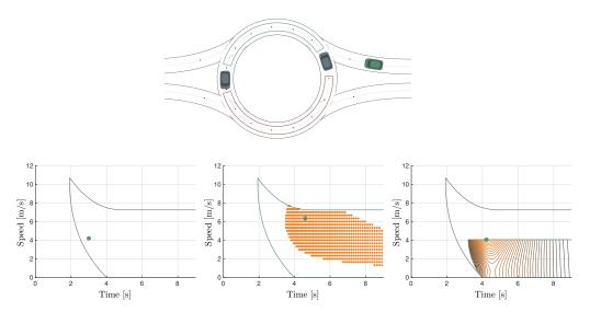
Figure 10.4 – At the top, a merging traffic scenario. At the bottom, three plots representing the decision-making process of the self-serving maneuver planner proposed in this thesis. In particular, plots at the bottom correspond, from left to right, to the: (i) reactive, (ii) explicitly cooperative, and (iii) predictive-reactive planners.
