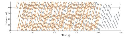
Figure 8.14 – Time-distance diagram representing the evolution over time of the vehicles in the circulatory lane, in the simulated scenario 16R1LR3L1I10-100V-2500Q[1 1 1]. The trajectories of R-Agents and PR-Agents are represented by ( — ) and ( — ), respectively.
