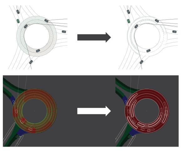
Figure 10.2 – Illustration of the contextual information provided by the proposed probably-free gaps. At the top, probably free gaps extracted in a simulated scene. At the bottom, the result obtained when the strategy is applied to a real data set.
