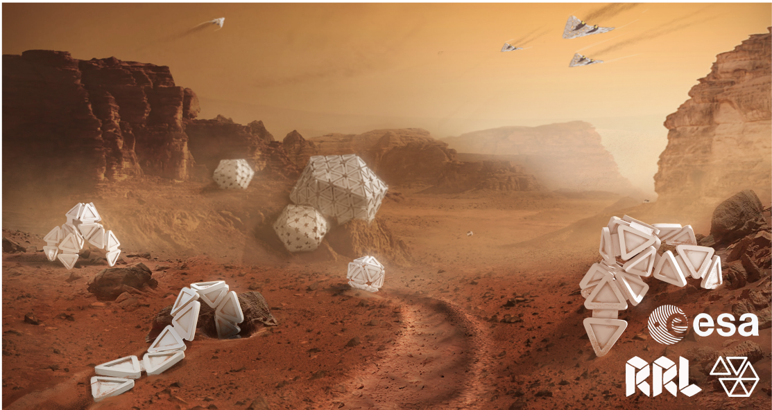
Figure 1.2 – Conceptual vision of the new paradigm in form of a universal extraterrestrial exploration system. A modular robotic structure based on polygons configures itself into a variety of mobile and structural assemblies such as domes, quadrupeds, snakes, and drones.
