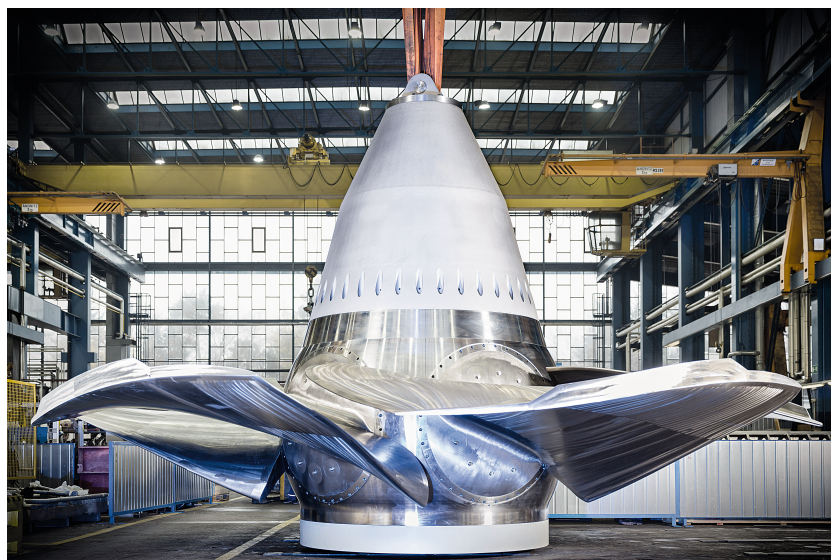
Figure 1.3 – Anti-cavitation lips on a Kaplan turbine runner manufactured by ANDRITZ HYDRO [81].
