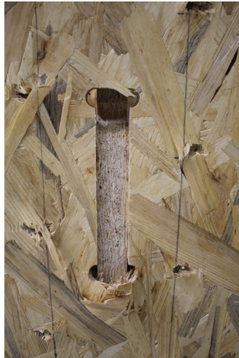
Figure 18: Failure by compression of wood fibers and slip
