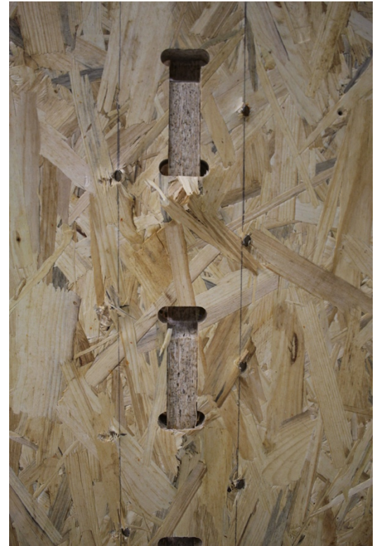
Figure 16: Failure by compression of the wood fibers
