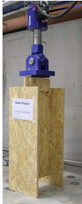
Figure 2: Standard testing setup, angled nailing sample
