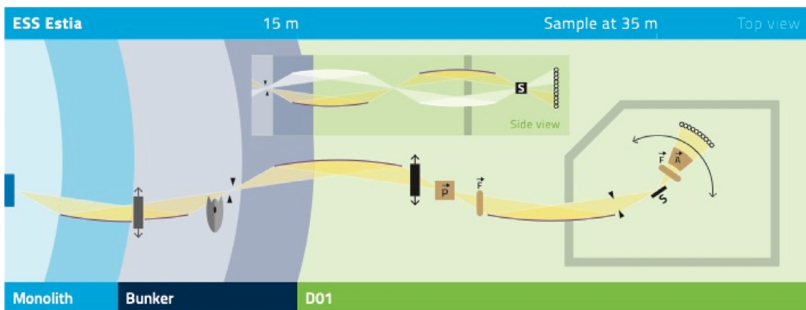
Fig. 11. Estia instrument layout. Components shown in white are foreseen upgrades.
