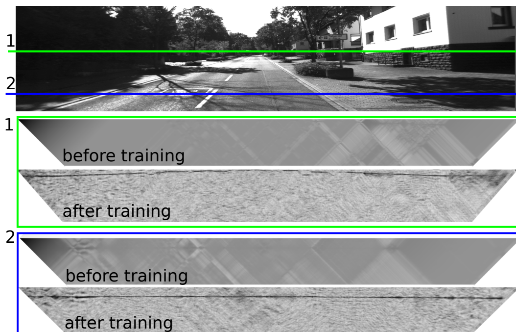
Figure 3.4 – Diagonal part of the matching cost matrices before and after the training with the MC-CNN-WS on the KITTI 2012 dataset. The top figure shows left rectified stereo image with two highlighted epipolar lines. The pictures below show the matching cost matrices for these epipolar lines. The dark elements in the cost matrices correspond to the lower cost. WTA error before the training is 42.01%, and 14.61% after the training. Note that before the training we can not visually distinguish the best matches in the cost matrices, while after the training they are visible.
