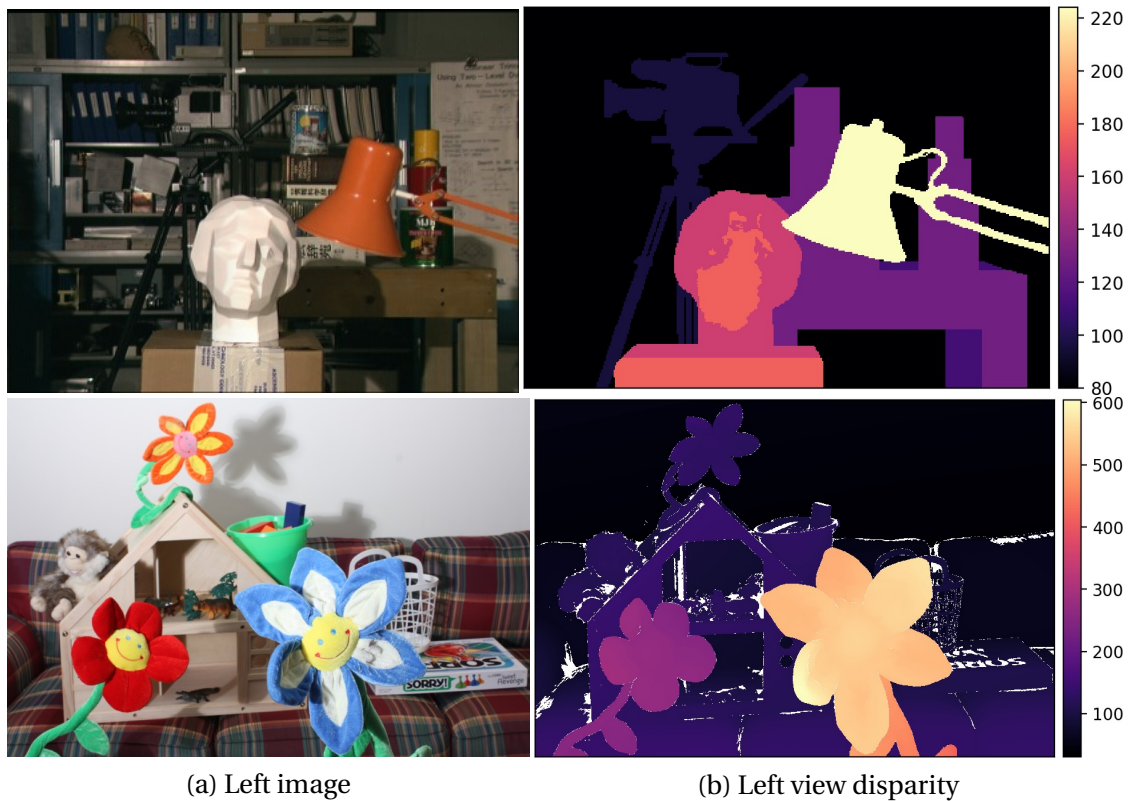
Figure 2.6 – Typical examples from the Middlebury dataset. In the disparity images, the white pixels correspond to the locations without the ground truth and the warmer colors correspond to larger disparities.
