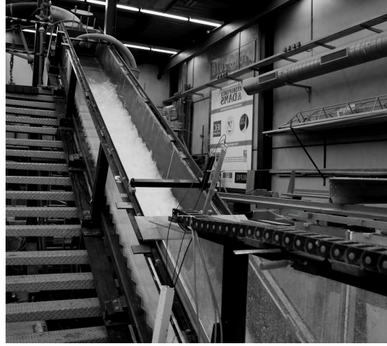
Figure 4.2 – Stepped chute flow characteristics seen from downstream for Run 10 (Table 4.1).
