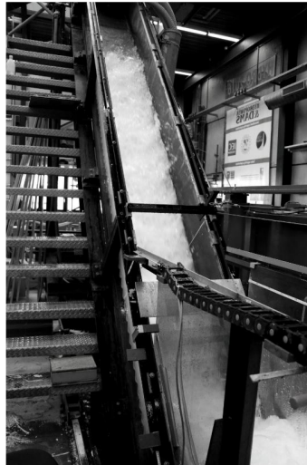
Figure 6.4 – 50° stepped chute flow characteristics seen from downstream for Run 26 (Table 6.1).
