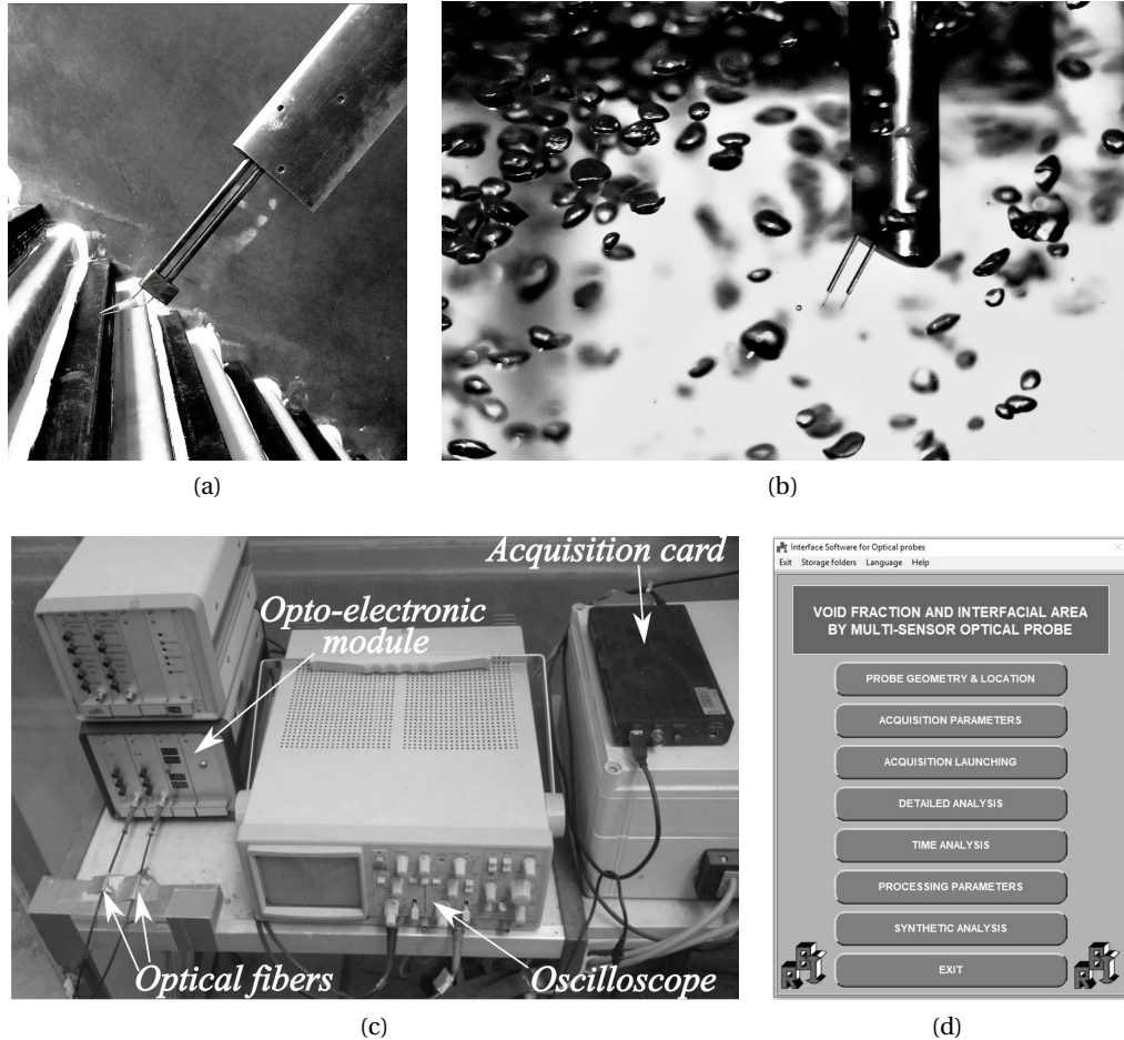
Figure 3.8 – The fiber optical phase detection system: (a) sideview of the FOP used for chute measurements, (b) sideview of the FOP used for stilling basin measurements in operation, (c) opto-electronic module, oscilloscope and acquisition card, and (d) acquisition and treatment software ISO v2.9.
