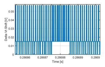
Fig. 5. Detailed view of 60us of the convolution kernel running. This view shows how the BTI-induced Vt shift varies over time, switching between relaxation periods, read and write phases.
