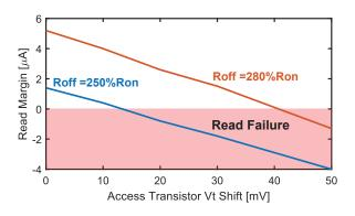
Fig. 2. Evolution of the read margin versus the BTI-induced Vt shift. A 250% ratio exhibits a 15mV maximum Vt shift before failure while a 280% ratio fails with 40mV of shift at 20 °C.
