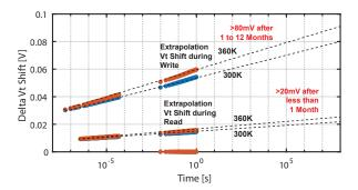
Fig. 3. Workload aware evolution of the Vt shift for the most used WL in the considered memory array at 20 and 80  $^\circ$ C. Linear extrapolation shows read failures happening after less than a month for a 250% HRS/LRS ratio. On the other hand, during write, more than 80mV Vt shift can be exhibited after less than a year.
