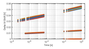
Fig. 4. Workload aware evolution of the BTI-induced Vt shift considering stochastic nature of the defect-centric BTI model [9]. Random creation/release of traps introduces variability in the aging process.
