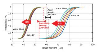
Fig. 1. Read current distributions for a 250% HRS/LRS ratio considering RRAM and CMOS variability at 20  $^{\circ}$ C. Distribution shift due to BTI-induced Vt degradation are shown and reduction of the read margin is highlighted (from black to red).
