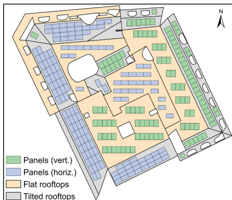
Fig. 3. Output of the virtual installation of PV panels after removing roof superstructures. The best configuration of vertically and horizontally oriented panels is selected. Panels on flat roofs are placed in south-facing rows and tilted at an optimal angle of 30°.
