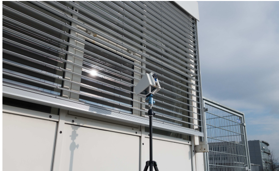
Figure 1. Set-up of the shading controller and Venetian blinds
