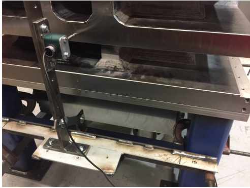
Figure B1.6 – Close up of LVDT positioned in the center of the middle rib, along the x -axis, with mounting bracket.
