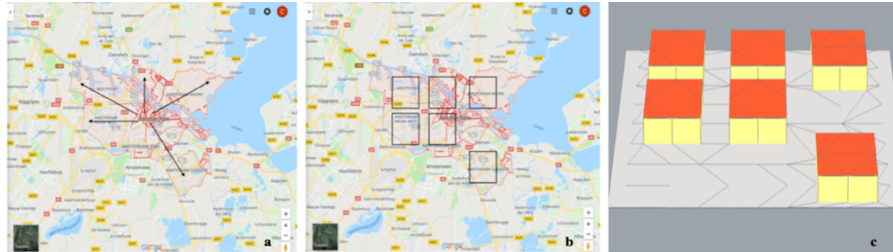
Figure 2. (a) Identification of the main urban development directions starting from the urban core (metropolitan area of Amsterdam) (b) Placement of a central building characteristic of the buildings of the urban centre, and of five adjacent buildings representative of the buildings in each direction of the urban development areas (given that Amsterdam is 30% built [9]), (c) Archetype imported into CitySim in the form of a DXF file.
