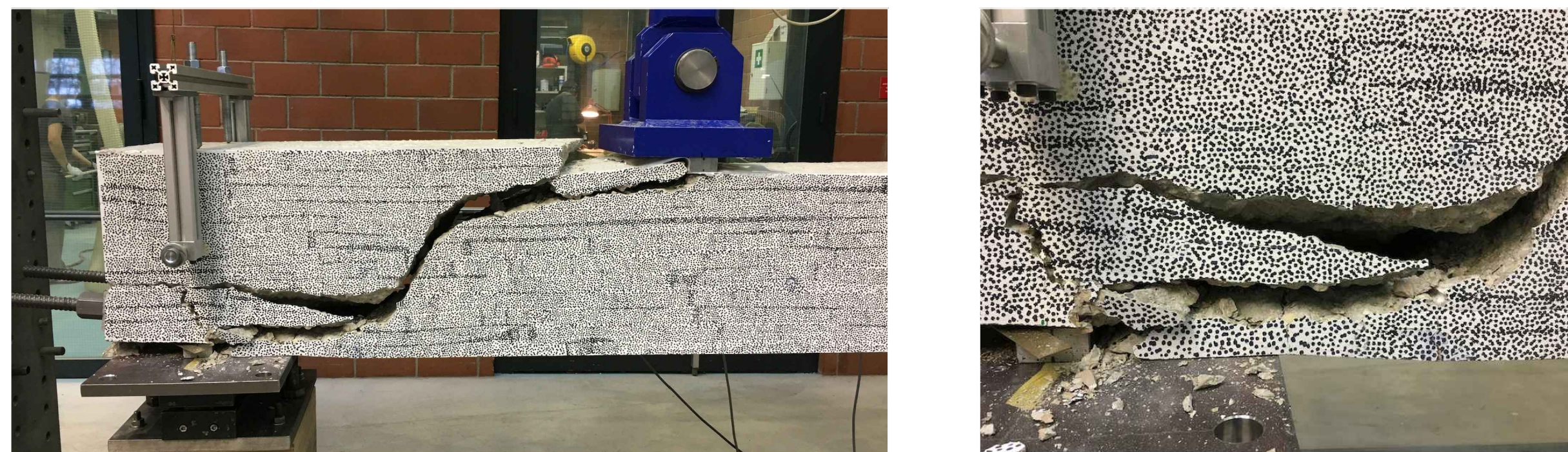
Figure 3: Post failure of sample SC75 showing very clearly the shear crack that led to the failure of the sample. On the right side a close up of the lower part of the fracture showing the influence of the dowel action on the failure mechanism.
