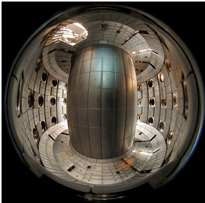
Figure 2.2 – Photograph of the inside of TCV, showing the graphite protection tiles that cover almost the entire vacuum vessel.
