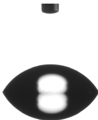
Figure 3.4 – Shape of a droplet deposited in CMI-processed SU-8 GM 1060.
