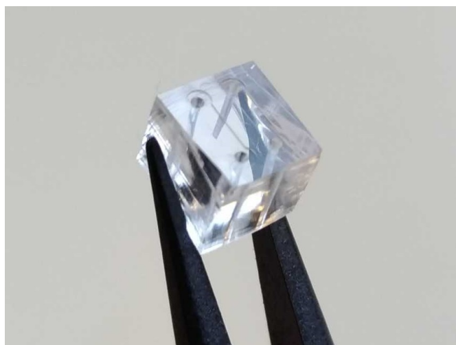
Figure 2.47 – PDMS stamp with microfluidic channels.
