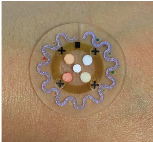
Figure 1.3 – Koh et al. Smart patch with four different selectively sensitive areas.
