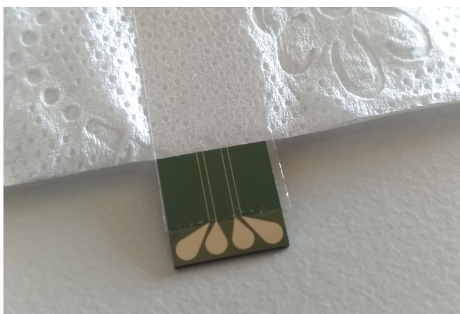
Figure 3.5 – Structure of the first prototype of the passive microfluidics. The channels here are represented by metal lines to be visible.
