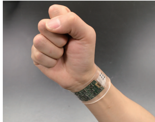
Figure 1.5 – Gao et al. Electrode-based FISA wristband.
