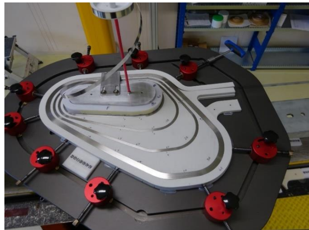
Fig. 5. First layer of GaToroid dummy prototype, wound in stainless steel tape on glass-filled nylon spacers (in white).
