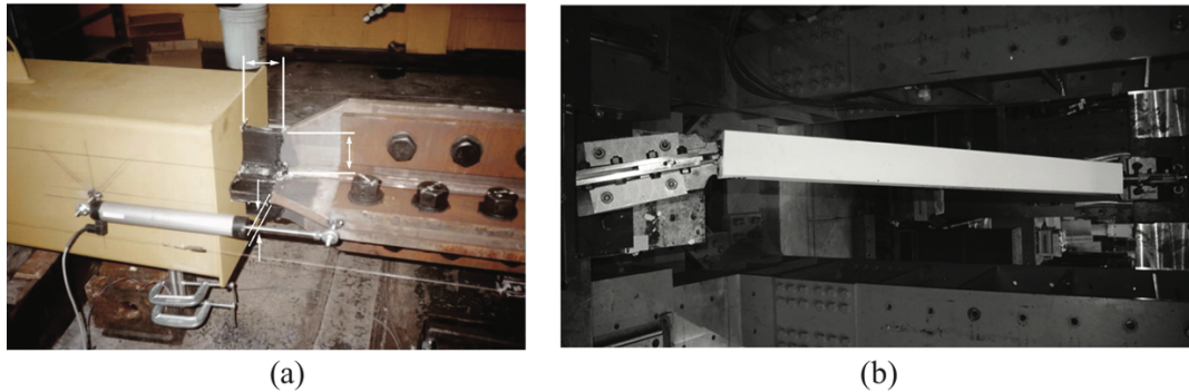
Figure 18. (a) brace at maximum deformation showing unsupported length (image adopted from Black et al. 2004b); (b) out-of-plane instability of the bracing connection (image adopted from Takeuchi et al. 2014a)
