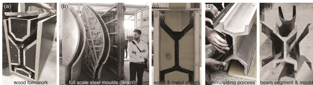
Figure 9. New formworking methods: a) classical wooden formwork, b) massive steel mould (Salvador de Bahia, Brazil), c) steel & wood mould assembly, d) demoulding, e) thin metal sheet formwork & beam segment.
