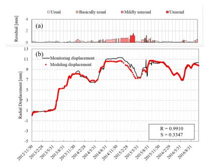
**Figure 8.** Time variation of (**a**) classified residual and (**b**) modelled and monitored displacement data for the monitoring point PL9-5.
