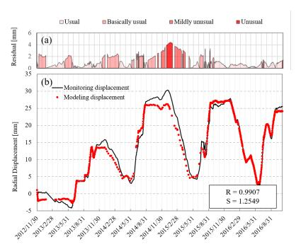
**Figure 6.** Time variation of (**a**) absolute residual and (**b**) modelled and monitored displacement data for the monitoring point PL9-3.
