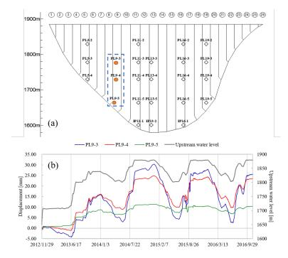
**Figure 5.** (a) Distribution of the monitoring points from upstream side view; (b) Time variation of radial monitored displacement data at the three selected monitoring points and upstream water level data.
