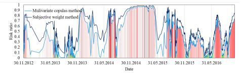
Figure 18. Multi-point risk ratios for dam Section 9# of the Jinping-I arch dam.
