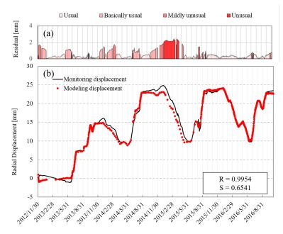
**Figure 7.** Time variation of (**a**) absolute residual and (**b**) modelled and monitored displacement data for the monitoring point PL9-4.
