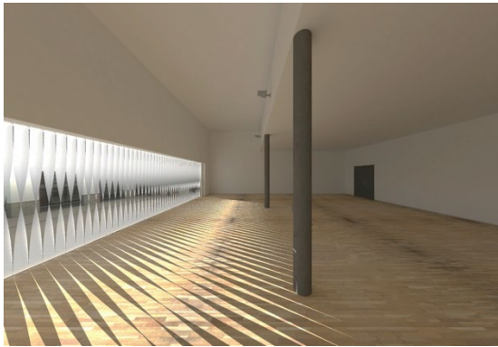
Figure 2. Example space simulated at 9:00 on March 15 th in sunny conditions with all slats tilted at 135°.
