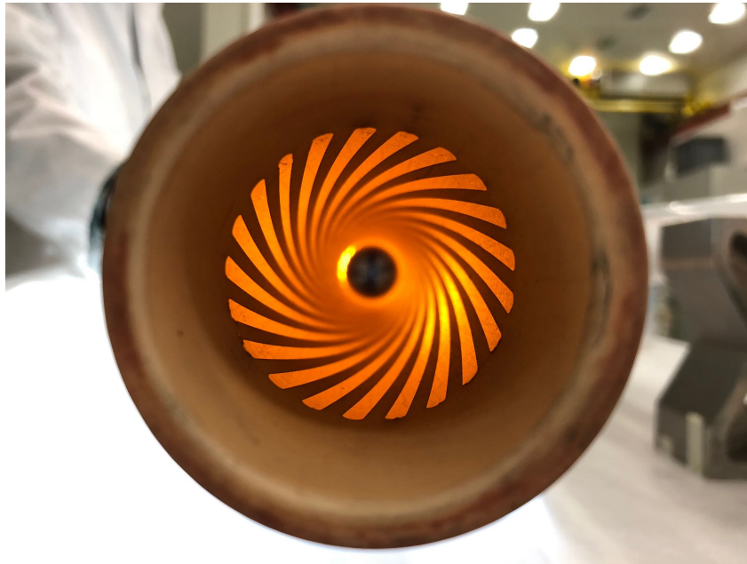
Figure 7.8 – Photograph of the prototype spiral beam screen with 21 screen conductors applied using Ag paint and \sim 4.5 turns along the length of the alumina tube installed in an LHC MKI.
