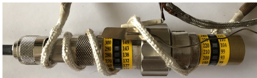
Figure 8.10 – Coaxial line test fixture with Dezifix terminated in short, PT100 temperature sensor, heating braid with temperature sensor and non-reversible temperature indicators.
