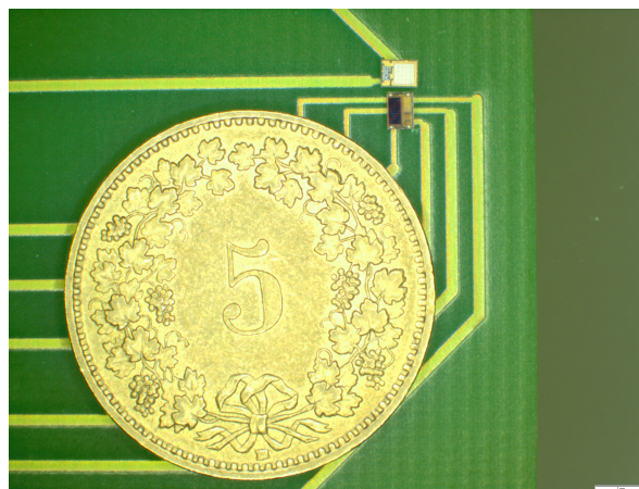
Figure 2.9 – The electronic components of the system with the photodiode (top) and photodetector (bottom).
