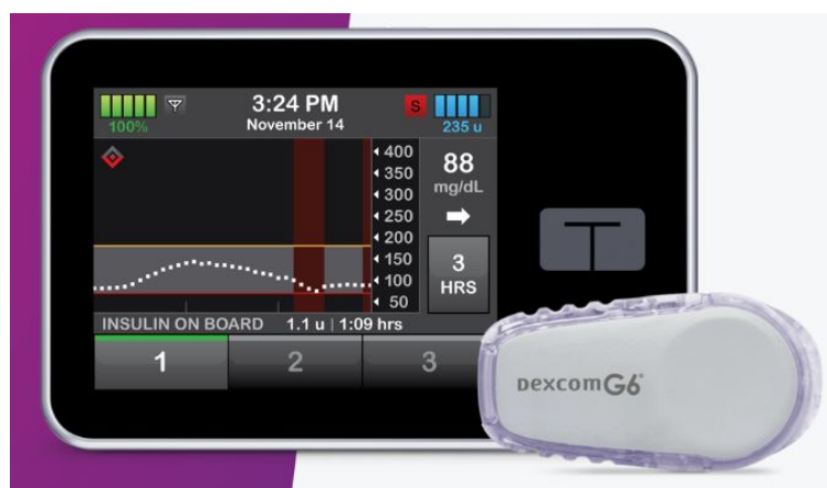
Figure 1.9 – t:slim X2™ Insulin Pump Predicts and helps prevent lows with Basal-IQ™ Technology [6]
