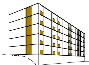
Figure 4.39 Schematic façade BIPV integration. AAF building scenario 2C.
