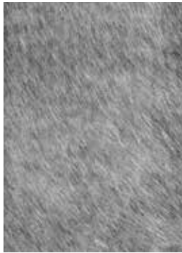
GLASS FIBRE generates 140-155 W/m 2
