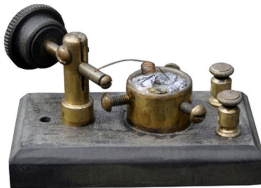
Figure 1.2 – A commercialized crystal detector introduced in early 1900s, picture courtesy of: John D. Jenkins, www.sparksmuseum.com .
