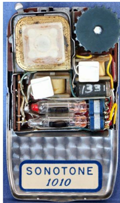
Figure 1.7 – The Sonotone hearing aid, the device contains one germanium transistor and two tubes, Courtesy of Bob McGarrah.
