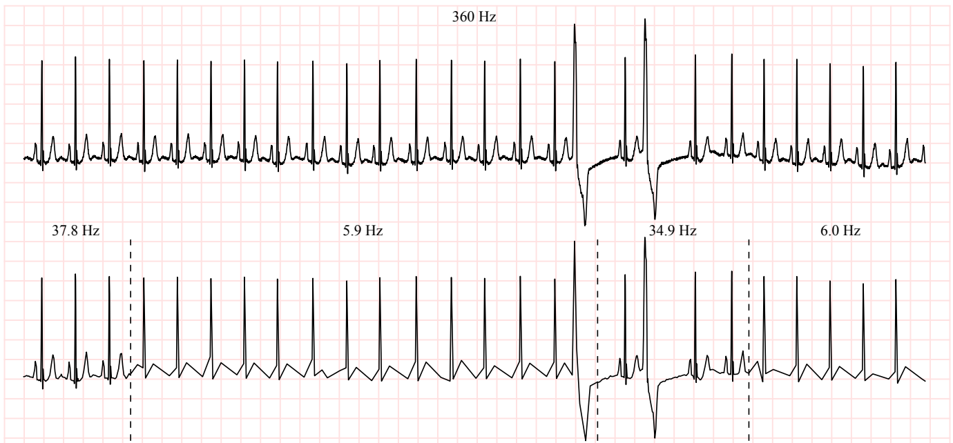
Figure 4: Event-triggered adaptive sampling of an ECG fragment using polygonal approximation. Top: Original signal, sampled at 360 Hz. Bottom: Resulting signal of the adaptive sampling method. The detection of a regular rhythm enables a substantial reduction of the sampling frequency by getting a much coarse representation of the signal. After a rhythm change (second vertical line), the sampling frequency is increased to allow getting the details of the abnormal area. [Source: Record 119 of the MIT-BIH Arrhythmia DB, lead MLII , between 17:10 and 17:24].
