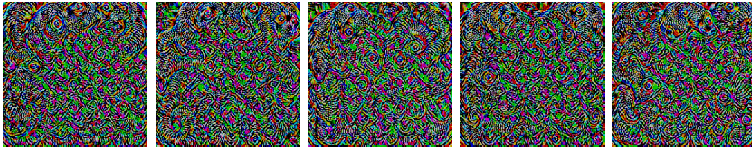
Figure 4.5 – Diversity of universal perturbations for the GoogLeNet architecture. The five perturbations are generated using different random shufflings of the set X . Note that the normalized inner products for any pair of universal perturbations does not exceed 0.1, which highlights the diversity of such perturbations.
