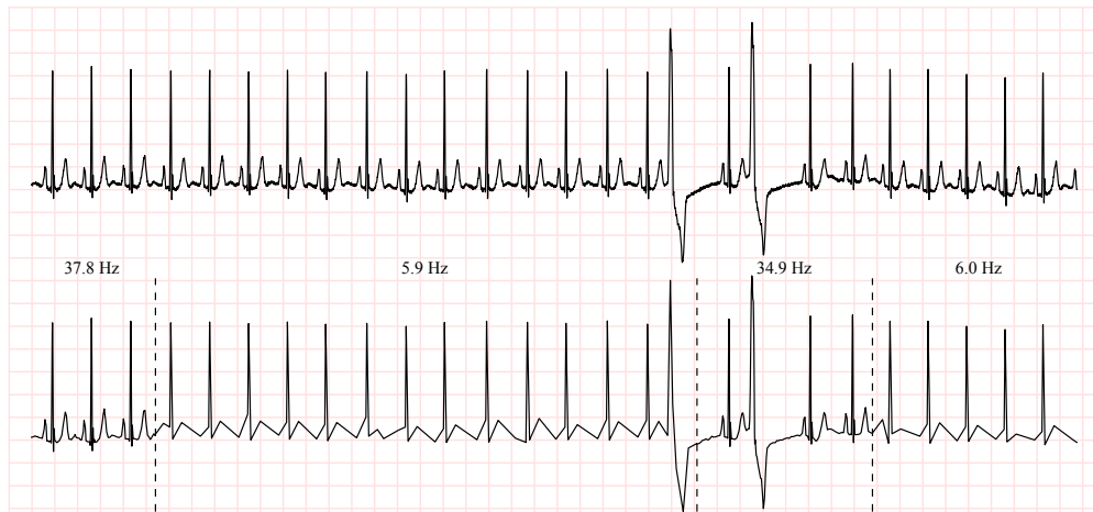
Figure 2.11 – Event-triggered adaptive sampling of an ECG fragment using polygonal approximation. Top: Original signal, sampled at 360 Hz. Bottom: Resulting signal of the adaptive sampling method. The detection of a regular rhythm enables a substantial reduction of the sampling frequency by getting a much coarse representation of the signal. After a rhythm change (second vertical line), the sampling frequency is increased to allow capturing the details of the abnormal area. [Data source: Record 119 of the MIT-BIH Arrhythmia DB, lead MLII , between 17:10 and 17:24]
