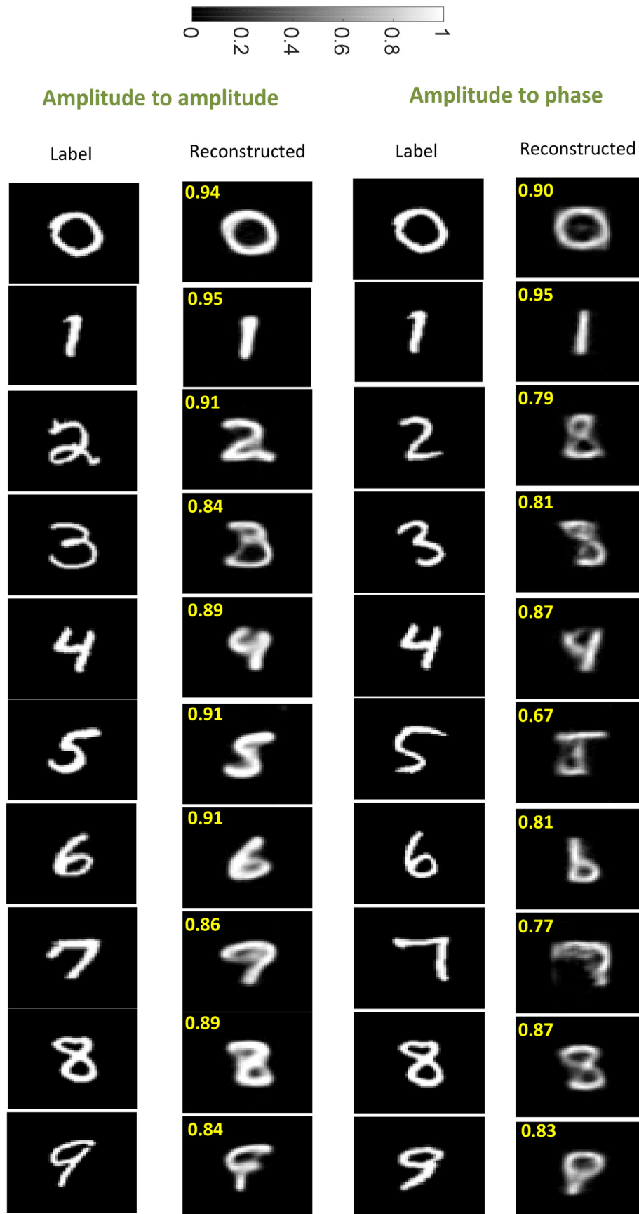
Fig. 6. Image reconstruction of speckle images corresponding to MNIST digit inputs to the MMF using DNNs.
