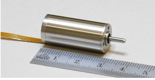
Fig. 1: The one-half inch diameter prototype used to validate the models in [3].
