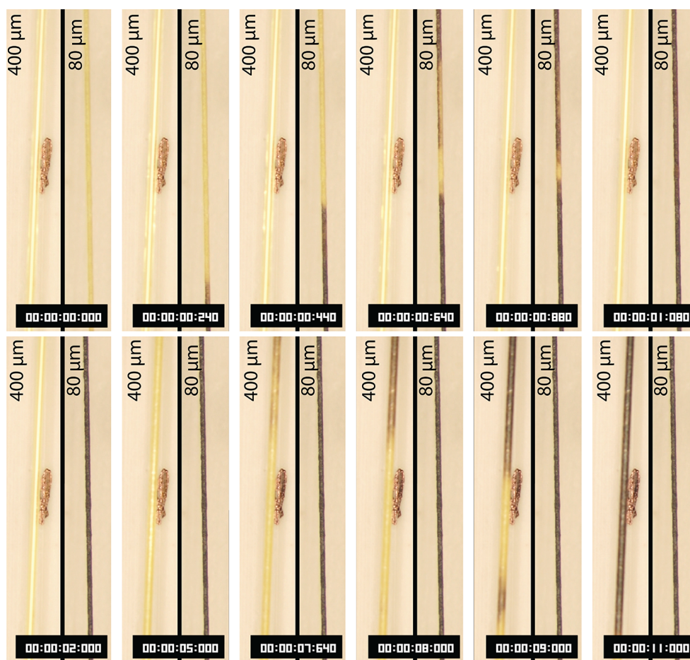
Figure 3.17 – Frame sequence showing the annealing process of MAPbI 3 on non-preheated substrates with diameters of 400 \mu\text{m} (left) and 80 \mu\text{m} (right). This sequence shows the marked differences in crystallization processes on the surfaces of substrates with 400 \mu\text{m} and 80 \mu\text{m} diameter, which occur much faster for the substrates with smaller diameter.
