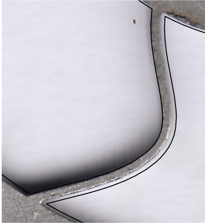
Figure 4.15 – Overlay of designed geometry in CAD and real geometry of membrane Var23 achieved by laser cutting
