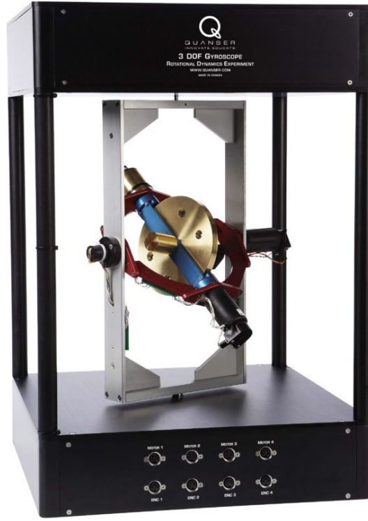
Figure 3.1 – The Quanser 3DOF Gyroscope used in the experiments.
