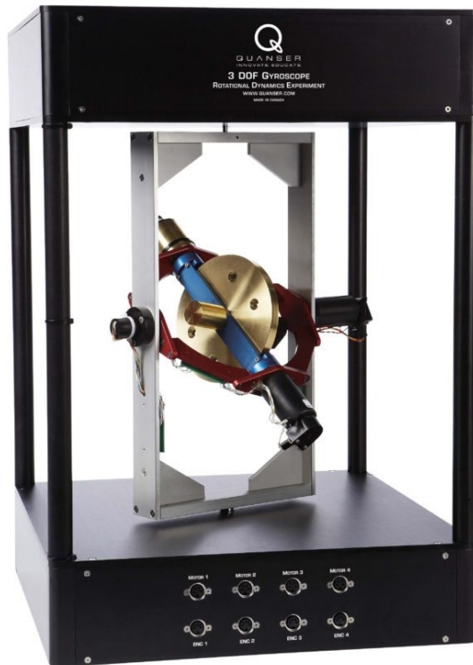
Figure 4.4 – The Quanser 3DOF Gyroscope used in the experiments.
