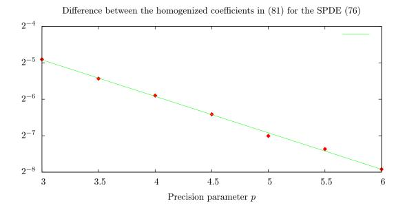
Figure 10: Error between the homogenized coefficients (see Eq. (81)) for the SPDE (76), as a function of the precision parameter p. The green line, obtained by polynomial fitting, has slope -1.01 in the  $p - \log_2(E_p)$  plane, which is close to the theoretical value of -1, showing a perfect agreement with the theory.
