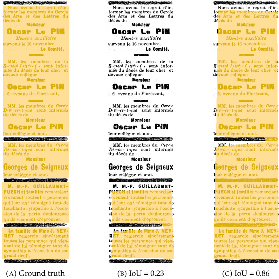
FIGURE 3.8: Example of the behaviour of the IoU metric. Figure 3.8a shows the pixels of the manual annotation (ground-truth). Figure 3.8b shows a bad prediction and thus the IoU is very low. Figure 3.8c shows a good prediction and thus the IoU is very high. The actual threshold at which an IoU is considered as good strongly depends on the practical use case.
