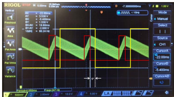
Fig. 3: Illustration of the synchronization signals: proj_{scan} , proj_{sync} , cam_{sync} .
