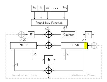
Figure 1: Block Diagram of Plantlet
