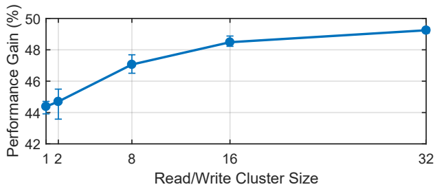
Figure 9: Performance gains of the RRAM-VAC while alternating reads and writes with bursts of different lengths for random inputs (addresses and data) versus burst size.
