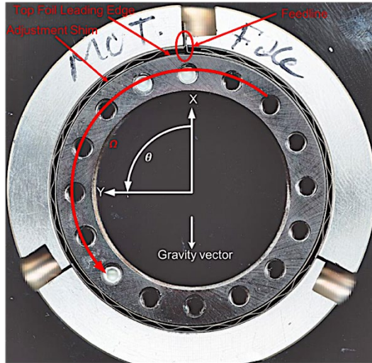
Figure 4 - Photograph of the actual test foil bearing under investigation highlighting the location of the feedline, the direction of rotation, and the angular reference.
