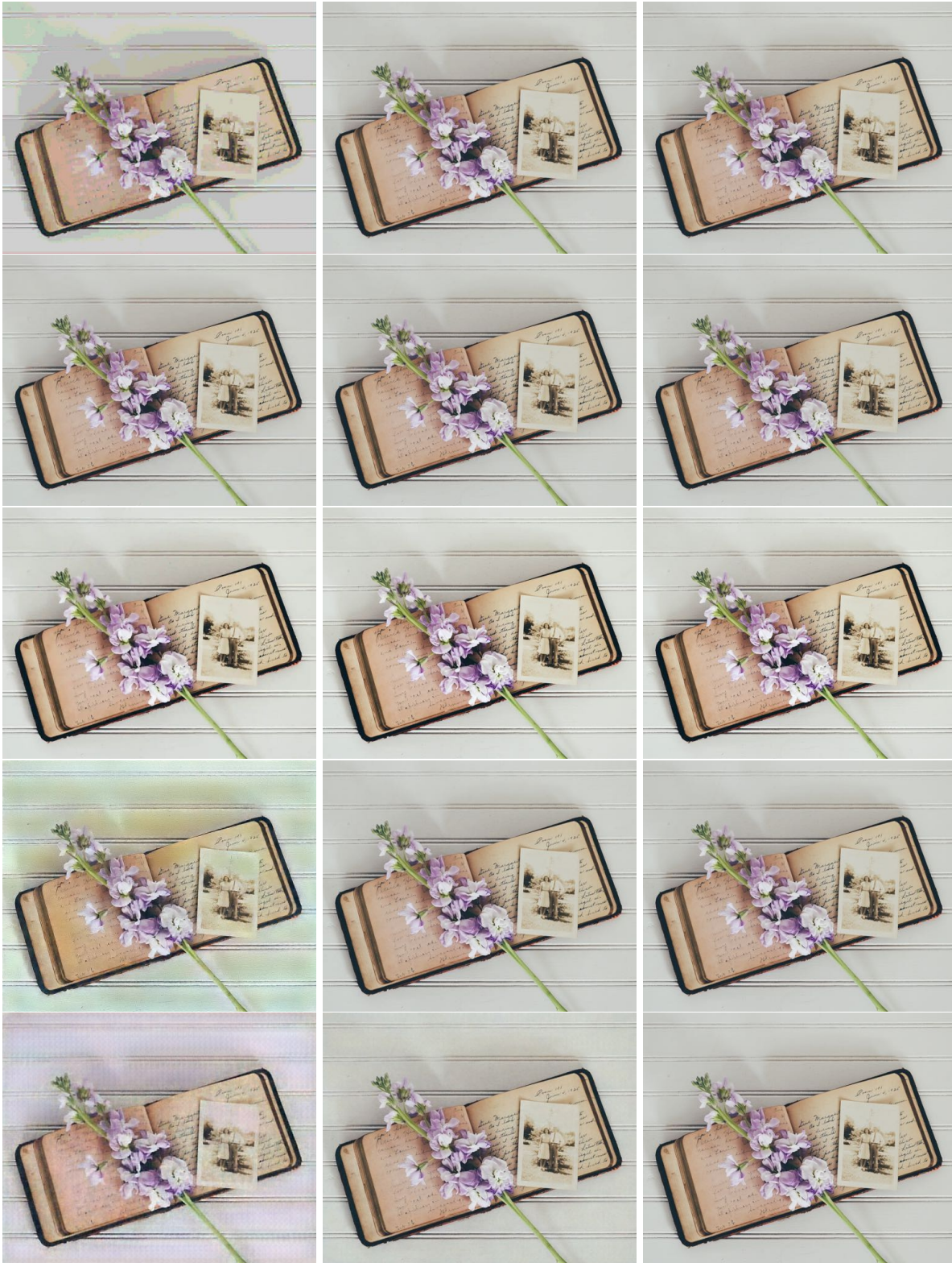
Figure 9: Reference image in Figure 5d compressed using JPEG, JPEG 2000, WebP, ResWCAE and ResMixWCAE from top to bottom, at target bitrates 0.12, 0.50 and 1.00 bpp from left to right, respectively.
