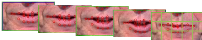
Figure 3.5 – Example of mouth boxes. Mouth region is detected based on landmarks. Features are computed in 3 \times 5 grid and grouped in a block of 5 frames.
