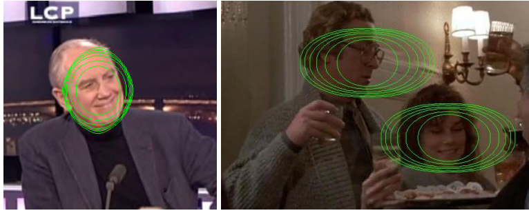
Figure 2.3 – Position. The different iso-contours of value 0 of the Potts costs for different values of \Delta (i.e. location of detections occurring after \Delta frames around each shown detection and for which \beta = 0 ), learned in an unsupervised fashion from TV REPERE (left) and Hannah (right). In the region delimited by a curve, association will be favored, whereas outside it will be disfavored. Curves show that more motion is expected on the Hannah movie, than on the TV data.
