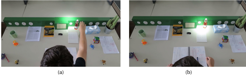
Figure 5.5 – User is pointing where the light is needed (a). Once the pose of Roombots spotlight is set, it remains on the desired location (b) as long as the user does not switch to the control mode.
