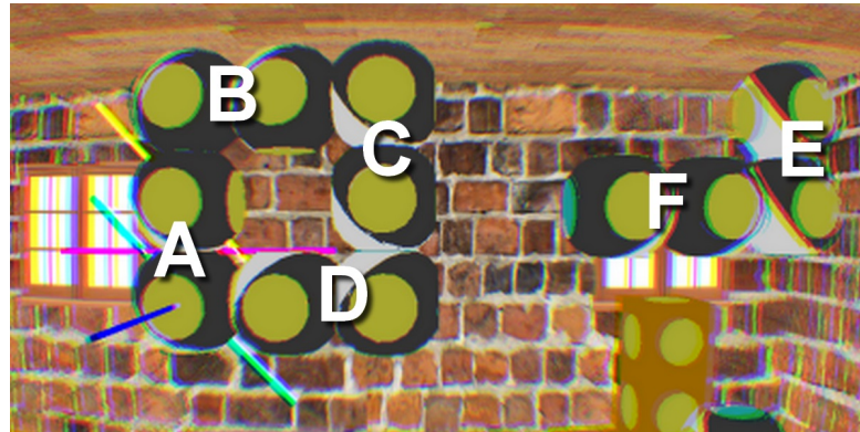
Figure 6.6 – On the left, a module loop forming a bulk. Module A is parent of B, which is parent of C which itself is parent of D. However, the chain stops here to avoid any infinite-update loop. D is thus parent of no module. Moving A would move the whole bulk, but moving C would only move D in addition. The same goes for any modification of configuration. On the right, a second bulk with E being the parent of F, hence the parent of this second bulk. If the user were to bring the left-hand bulk close-enough to F, the whole bulk would be snapped, but no connection would be made (even though the connector of F is active, as shown by its pale blue color). Indeed, after this connection, it is unclear which module becomes the parent of all modules.
