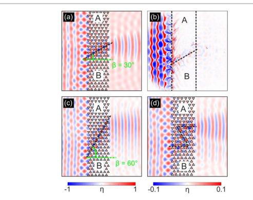
**Figure 4.** Water wave fields obtained for different geometries of interfaces at 22 Hz. (a) Numerical simulation and (b) experimental transmission of a 30° interface. (c) Numerical simulation of a 60° interface and (d) Numerical simulation of a zigzag shaped interface.
