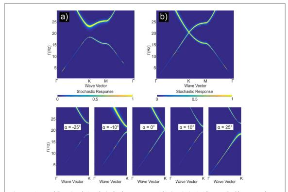
**Figure A2.** Computed dispersion relations obtained as the response to a stochastic excitation [45] for a water level h=7.3 mm for  $\alpha=30^\circ$  in (a),  $\alpha=0^\circ$  in (b). In the lower row of panels, 5 different angles are used and only the Brillouin zone direction of interest, i.e.  $\Gamma$  K is depicted.
