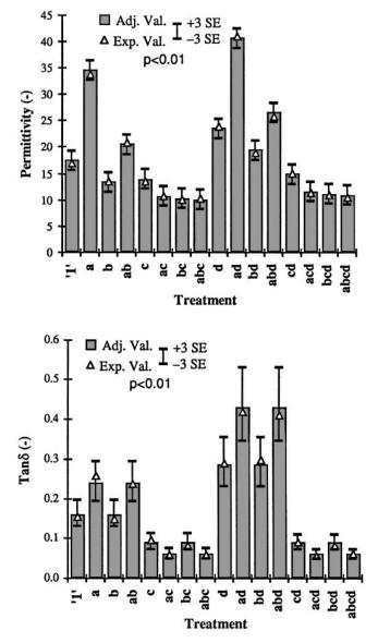
FIG. 7. Control chart of results of experimental plan used to assess the effect of various parameters on the dielectric properties of different vermiculite films.
