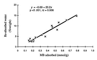
FIG. 5. Plot of water readsorption versus quantity of methylene blue adsorbed for various vermiculites.
