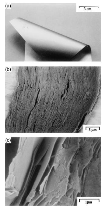
FIG. 2. Images of K-Bu vermiculite film: (a) typical flexible film, (b) typical transverse section, and (c) rupture surface.
