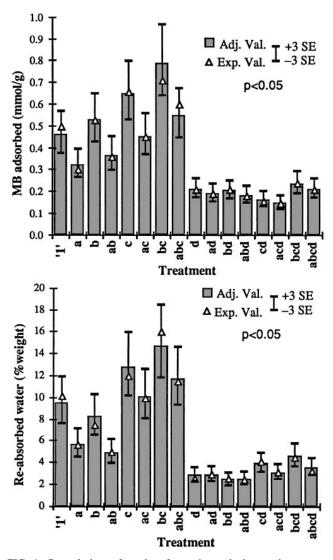
FIG. 4. Control chart of results of experimental plan used to assess the swelling, delamination, and water affinity of various vermiculite films (SE: standard error).
