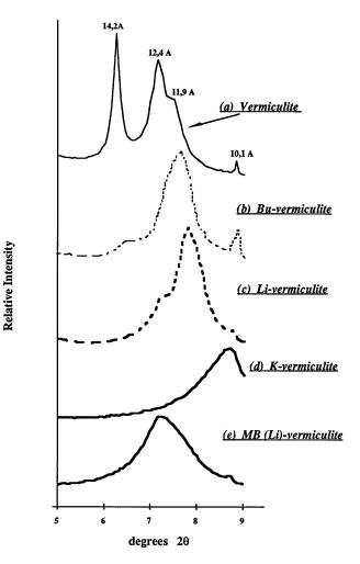
FIG. 1. X-ray diffractograms for the starting vermiculite and different vermiculite films: (a) exfoliated starting material, (b) Bu vermiculite, (c) Li vermiculite, (d) K (Li) vermiculite, and (e) MB exchanged (Li) vermiculite.
