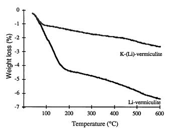
FIG. 6. Thermogravimetric analysis curves for Li vermiculite and K (Li) vermiculite films.
