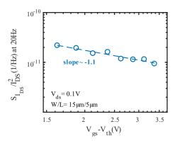
Fig. 5 Normalized drain current noise power spectral density against overdrive voltage  $(S_{DS} / I_{DS}^2)$  versus  $V_{gs} - V_{th}$ ) at a frequency of 20 Hz for a TFT biased in the linear regime. The extracted slope, m  $\approx -1.12$ , indicates that the 1/f noise follows the carrier number fluctuation theory with correlated mobility fluctuations.
