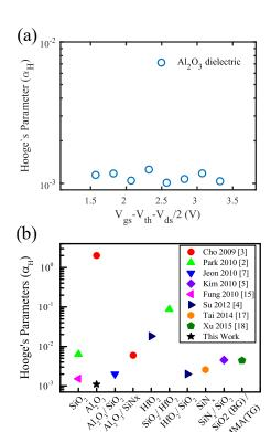
Fig. 4 (a) Extracted Hooge's parameter as a function of  $V_{gs}$ - $V_{th}$ - $V_{ds}/2$  for a-IGZO TFTs with a 20 nm Al<sub>2</sub>O<sub>3</sub> gate dielectric. (b) Reported Hooge's parameter for a-IGZO TFTs with various gate dielectrics. For devices with a bilayer of gate dielectrics, the dielectric in contact with the channel is mentioned in second place. For the last device, BG and TG correspond to back-gate and top-gate respectively.
