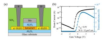
Fig. 1 (a) Schematic cross-section of the fabricated top-gate self-aligned (SA) a-IGZO TFTs with  $Al_2O_3$  gate dielectric, (b) Transfer characteristics,  $I_{DS}-V_{GS}$  curve, in linear regime ( $V_{DS}=0.1$  V) for W=15  $\mu m$  and L=5  $\mu m$ .
