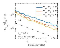
Fig. 2. Normalized drain current noise power spectral density  $(S_{ID}/I_{DS}^2)$  of a TFT biased in the linear regime for different  $V_{gs}-V_{th}$ .
