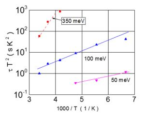
Fig. 6. Arrhenius plot obtained using noise spectra measured at different temperatures for the sample with L = 1200 nm.
