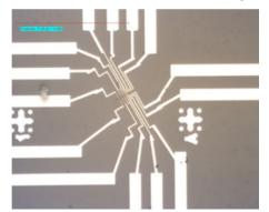
Fig. 1. An optical image of an InAs nanowire chip.
