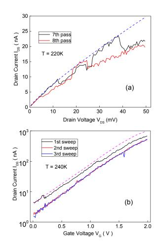
Fig. 2.  $I_D(V_{DS})$  dependences of the sample with L = 3 µm at two gate voltages (a)  $V_G = 0$  and (b)  $V_G = 2$  V as well as at different temperatures in the range from T = 100 K to T = 297 K. The change step is  $\triangle V_{DS} = 0.5$  mV. The curves are smoothed by the Savizky-Golay method, a second-order polynomial, and the window length is 15 points. The dashed line indicates a linear relationship.
