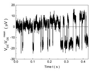
Fig. 4. Time trace demonstrating RTS behavior in the drain current of an NW sample (L = 3  $\mu$ m), V<sub>DS</sub> = 20 mV, V<sub>G</sub> = 0, T = 220 K.
