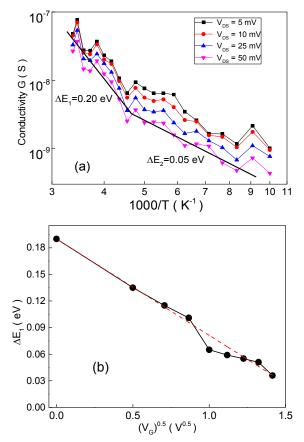
Fig. 5. (a) Temperature dependences of the conductivity of InAs NW with a length of L = 3  $\mu$ m at  $V_G$  = 0 and several voltages of  $V_{DS}$  (indicated in the inset). (b) The dependence of the activation energy  $\Delta E$  as a function of  $\sqrt{V_G}$ , obtained for  $V_{DS}$  = 50 mV. The dashed line indicates the calculated dependence obtained in accordance with Eq. (1).
