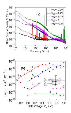
Fig. 7. (a) Noise spectrum of sample 5 (L = 600 nm),  $V_{DS} = 10$  mV,  $V_G = -0.3$  V to +0.1 V, T = 150 K; (b) the low-frequency Lorentzian noise plateau values,  $S_I$  (0), extracted from measured noise spectra, as a function of gate voltage, T= 300K. The inset shows a schematic of the band structure with quantum levels of 1D conductivity in an NW structure.
